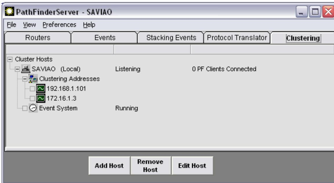
This picture shows the name of the machine on which PathfinderPC Server is running and the various NIC cards that are in the system. By default, all of these NIC cards are enabled for clustering communications. Selecting the host name and clicking edit allows these settings to be fine-tuned.
