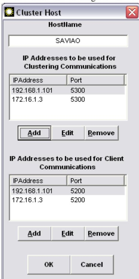
Using this screen you can define which NIC cards are to be used for clustering communications and the order in which they will be used. You can also define which of the NIC cards can be used for copies of the PathfinderPC Mini or Client to communicate with the server.
